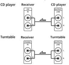
• If your turntable has an earth lead To prevent hum, connect the earth lead to the  $\frac{1}{2}$  ground terminal on the receiver.
